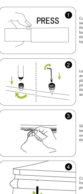
Connect frame sections by pressing the spring loaded buttons and sliding the two parts together.
